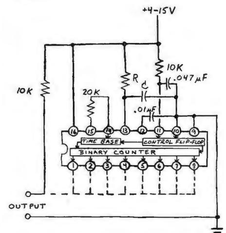
Fig. 1. Schematic of XR-2240 in free-running (astable) mode.
